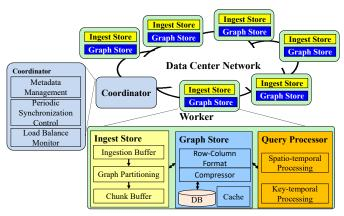
Fig. 2. PAST system architecture.
