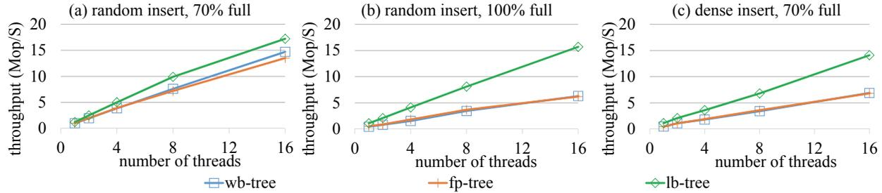
**Figure 12: Insertion performance varying the number of threads from 1 to 16.** (We bulkload a tree with 2 billion (8B key, 8B value) entries 70% or 100% full. Then every thread performs 100K random insertions, or a different group of 100K dense insertions.)
