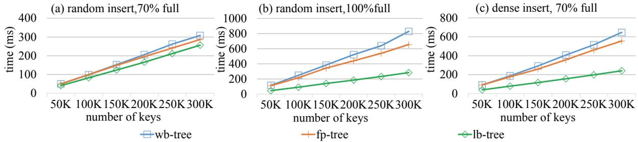
**Figure 11: Insertion performance varying the number of operations.** (We bulkload a tree with 2 billion (8B key, 8B value) entries 70% or 100% full, then perform 50K–300K random insertions, or dense insertions to the right-most leaf node in a single thread.)
