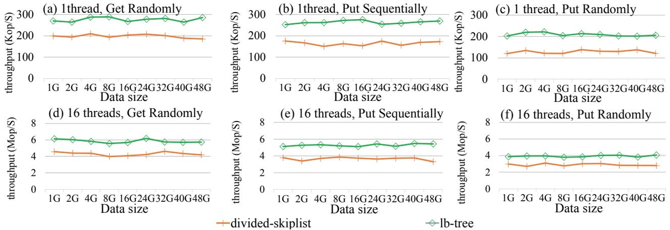
**Figure 16: X-Engine performance with LB<sup>+</sup>-Tree vs. skip list.** (Before the experiments, we bulkload an index to have 1GB, 2GB, ..., 48GB data. Then we perform 100K Get operations randomly, 100K Put operations sequentially, or 100K Put operations randomly in every thread. We use *db.bench* to produce (8B key, 20B value) entries. The number of threads is either 1 or 16.)
