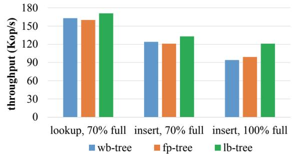
**Figure 17: Memcached performance with three B<sup>+</sup>-Tree structures as its core index.** (We bulkload a tree with 50 million entries 70% full or 100% full, and use *mc-benchmark* to get (lookup) or set (insert) 500K random keys. The keys are 20-byte random strings.)
