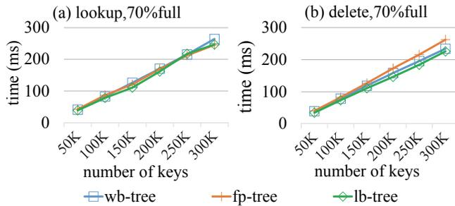
**Figure 14: Search and deletion performance varying the number of operations.** (We bulkload a tree with 2 billion (8B key, 8B value) entries 70%, then perform 50K–300K random search or deletion operations in a single thread.)
