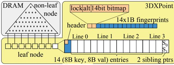
Figure 4: The LB<sup>+</sup>-Tree structure with 256B nodes.
