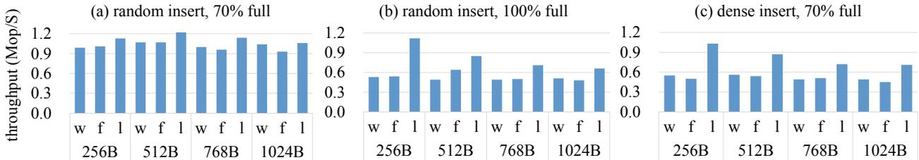
**Figure 13: Insertion performance varying node size.** (We bulkload a tree with 2 billion (8B key, 8B value) entries 70% full, then perform 100K random back-to-back insertions in a single thread. w: wb-tree, f: fp-tree, l: lb-tree.)
