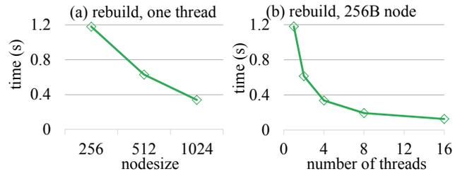
**Figure 15: Non-leaf rebuild time during recovery.** (During recovery, leaf nodes contain 2 billion (8B key, 8B value) entries 70% full. We vary the node size and the number of threads for rebuilding the non-leaf nodes.)
