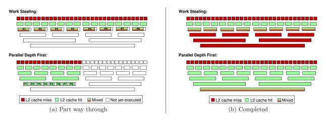
Figure 1: Scheduling parallel Mergesort using WS and PDF: Picturing the misses. Each horizontal box is a sorted array of records, where at each level, pairs of arrays from the previous level are merged until all the records are sorted. The L2 hits and misses are shown for sorting an array of  $C_P$  bytes, where  $C_P$  is the size of the shared L2 cache, using 8 cores.
