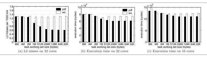
Figure 6: Varying the task granularity of parallel Mergesort for default configurations.
